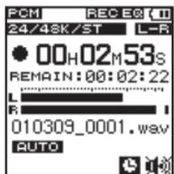
When recording starts, the **REC** indicator lights, and the elapsed recording time and the remaining recording time are shown on the display.
