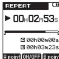
By default, the repeat starting point (A) is set at the beginning of the file and the ending point (B) is set at the end of the file. If you want to repeat the playback of an entire file, press the **+** key without changing the A and B points
