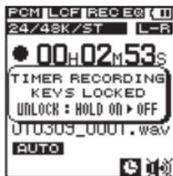
If you want to operate the unit during timer recording, slide the **⏻ / |/HOLD** switch toward the **HOLD** position momentarily to disable the hold function.
