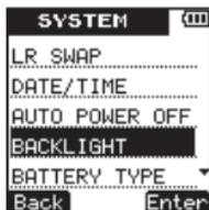
5 Press the ►► (Enter) key to open the BACKLIGHT setting screen.
